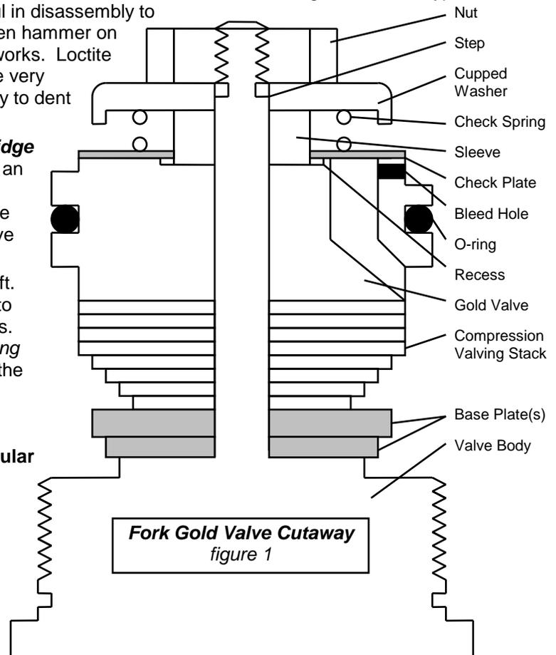
6 If your Custom Setup requires a Compression Bleed Hole - Drill one hole horizontally, through one of the port walls just above the step for the o-ring on the Compression Gold Valve. Placement is not critical. If your application is Racing please use the Bleed Hole size recommended in the Valving Notes section of the DVS Custom Setup Sheet.
